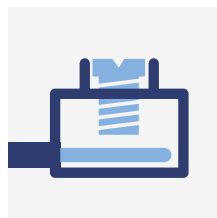
Loose screwed connections
